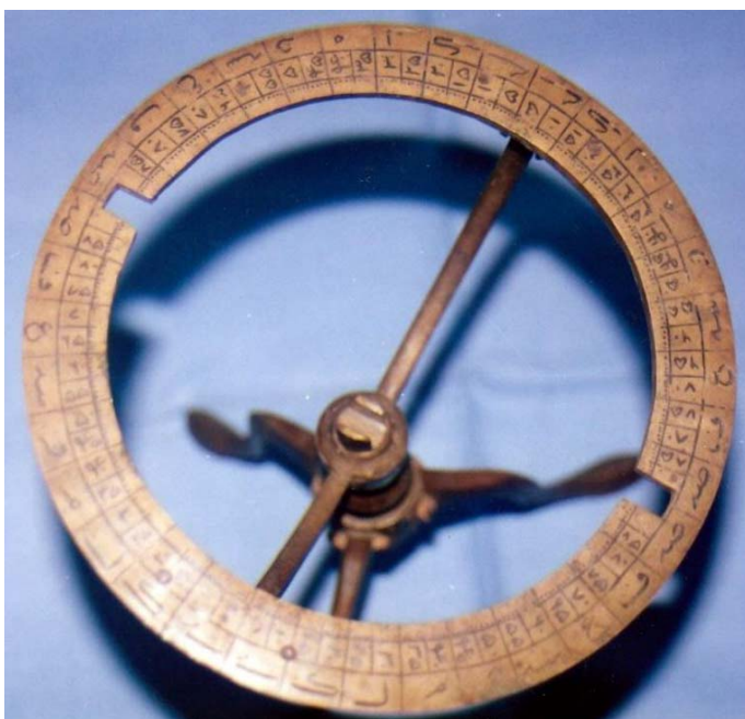
Fig. 4. An example of a horizontal circle, inside of which a celestial globe was installed. All three grooves into which the vertical circle was placed are visible [14, P. 3067].
